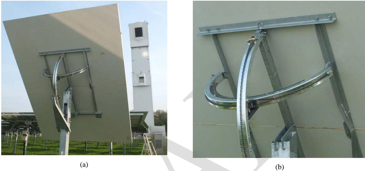
**FIGURE 5.** (a): First rim drive prototype with 8 m<sup>2</sup> mirror surface mounted at Solar Tower Jülich, Germany (without drive units); (b): Detail.
