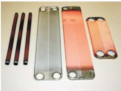
New enhanced evaporator surfaces manufactured by vacuum plasma spray
