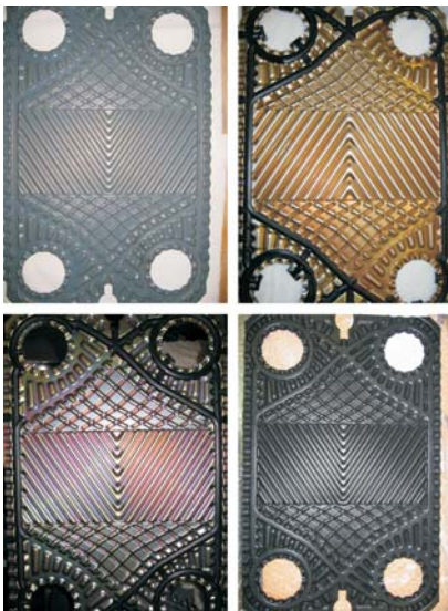
New enhanced evaporator surfaces manufactured by vacuum plasma spray
