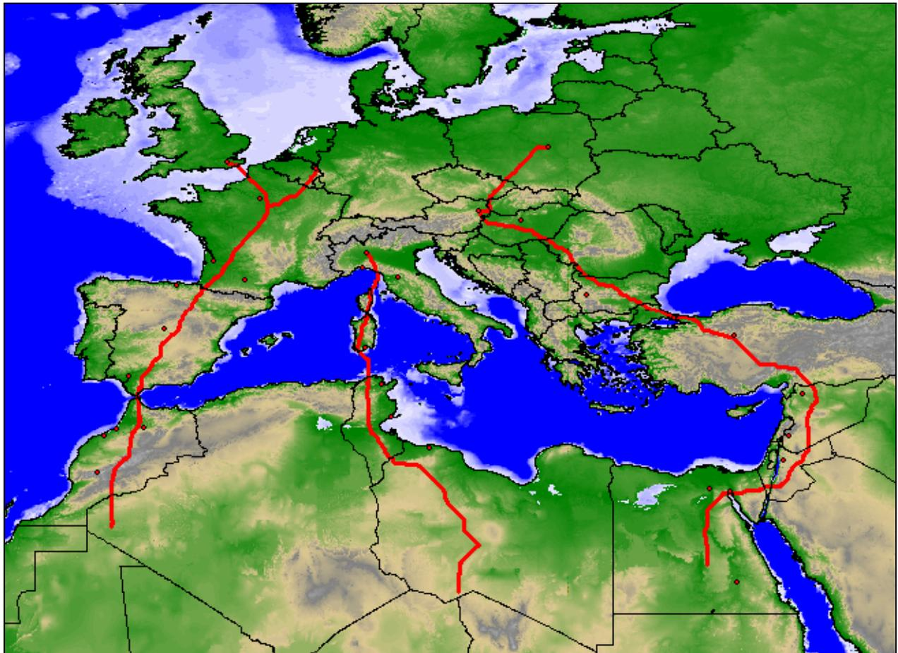
**Figure 5-8: Three analysed samples of EUMENA interconnections with HVDC lines with a capacity of 5 GW each. The red dots indicate further centres of demand that are close to the line and could be interconnected, too. The background map shows the topographic features of the landscape /May 2005/**
