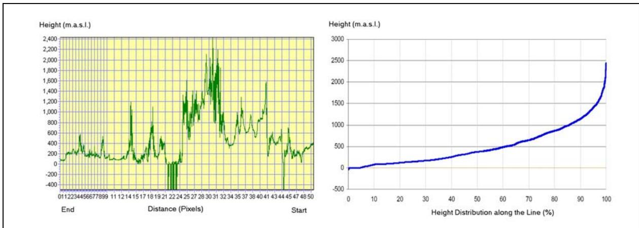
**Figure 5-11: Ground profile (height above sea level) of line 3 from Central Egypt to Warszawa, Poland and the associated hypsographic elevation model.**
