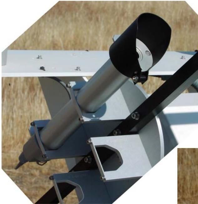
pointing in exact direction to the sun. An additionally shadow ball is fixed on the sun tracker in that way that it is always shading the DHI sensor. The two pyranometers of course always stay horizontally mounted.
