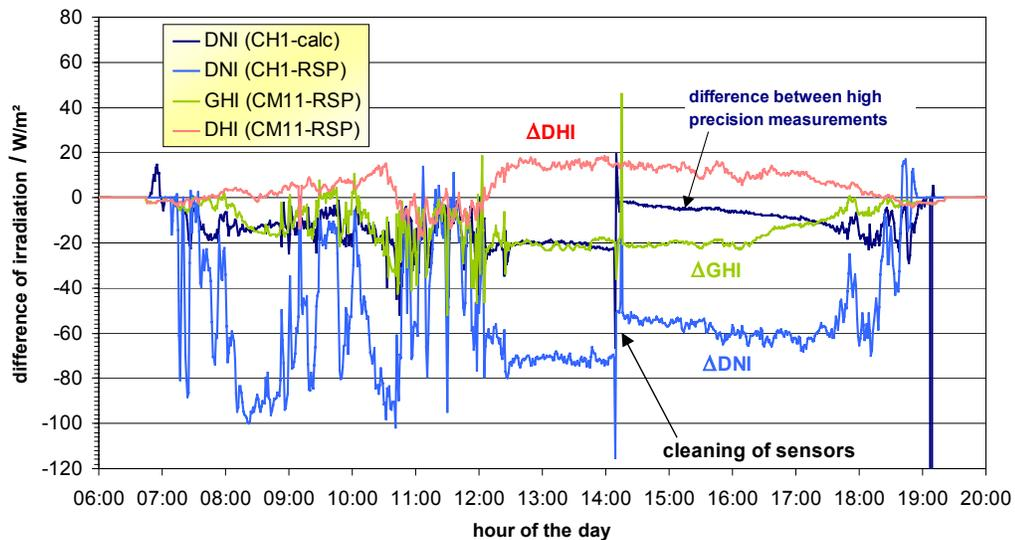
The difference of the DNI of the high precision instruments lies beyond 20 W/m<sup>2</sup> what means an accuracy in deviation of less than 4 %. At 14:10 a sudden break down of the deviation to only a few W/m<sup>2</sup> can be seen: this is caused by cleaning the sensors after a 6 days pe-
