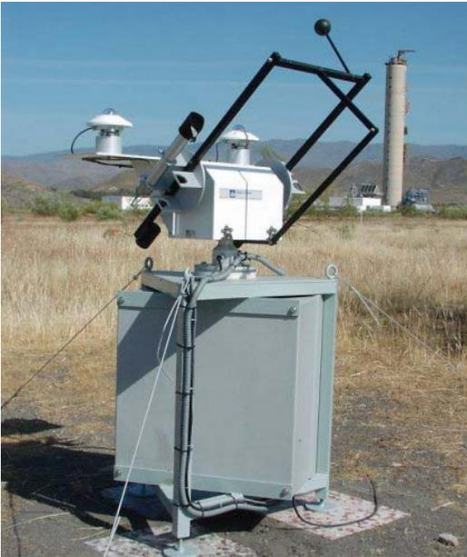
*Figure 1: Rotating Shadowband Pyranometer (RSP) in normal position (left) and during rotation (right).*
