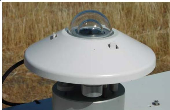
nificant part of the near infrared solar radiation is absorbed by water vapor. Calibration of the RSP Radiation Sensor has been carried out by the manufacturer against an Eppley Precision Spectral Pyranometer (similar to our Kipp&Zonen pyranometers) for 3 to 4 days under daylight conditions. Depending on the exact sky conditions during that period there also may exist a certain error of the determined calibration constant.
