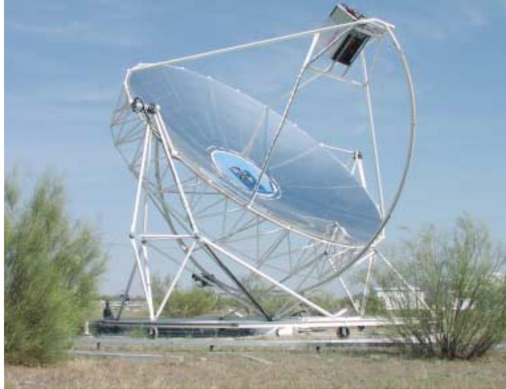
**Figure 6** The EURO-DISH parabolic dish concentrator with a Stirling motor-generator in the focal point at the CIEMAT solarthermal test centre Plataforma Solar de Almeria, Spain (Source: SBP)
