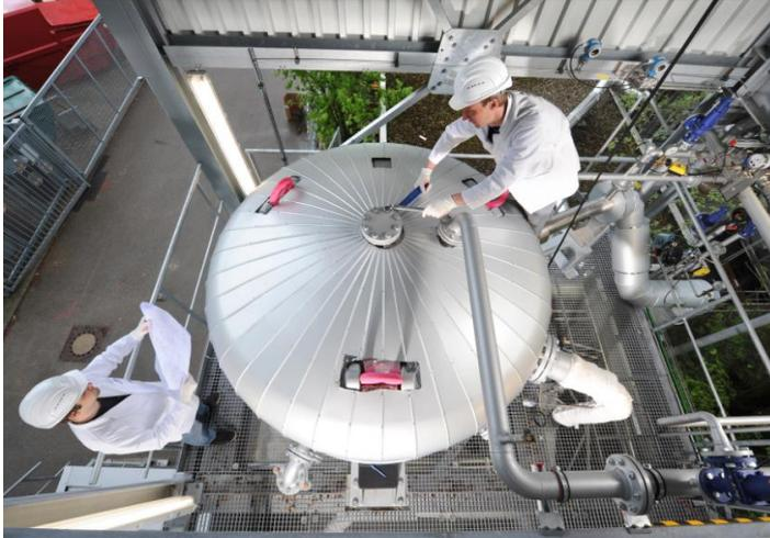
Fig. 5: DLR HOTREG test facility for regenerator and packed bed storage types with pressurized air up to 800°C and 10 bar.
