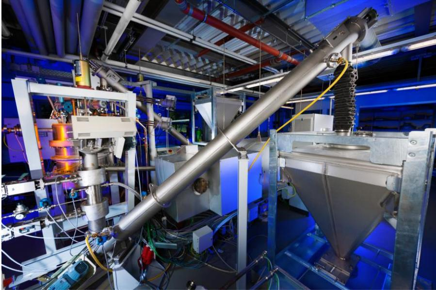
Fig. 8: DLR TCS-test facility for thermochemical storage based on quick lime and water.
