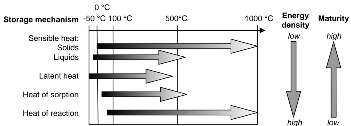
Fig. 1: Thermal energy storage mechanism, their working temperature, and correlation to energy density and status of technical maturity.
