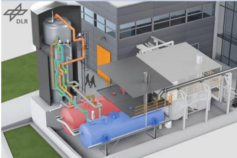
Fig. 6: DLR test facility for thermal energy storage in molten salt (TESIS) – TESIS:store - storage test section for thermocline-filler one tank concept.
