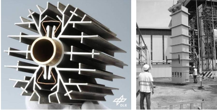
Fig. 7: Photos of steam/water containing steel tube with aluminum fins to enhance heat transfer (left, figure without PCM in between the fins) and DLR prototype PCM-storage module (right, figure shows storage module without insulation).
