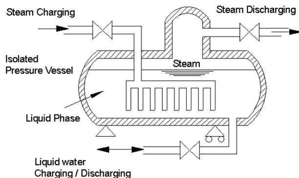
Fig. 3: Scheme of a steam accumulator for sensible heat storage in pressurized water.
