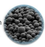
Aerogels are highly porous solid materials with low densities and low thermal conductivities synthesized via sol-gel processing.
