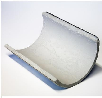
Fiber-reinforced silica aerogel for thermal insulation and shielding
