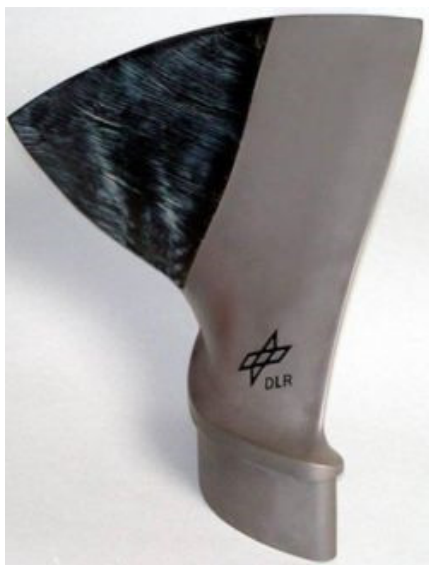
Hybrid demonstrator fan-blade, which is composed of a CFRP fan bladed bonded to Ti-6Al-4V
