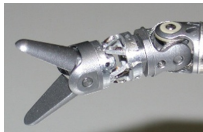
Fig. 2: Tiny gripper for surgical operations
