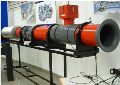
Fig. 9: Flow passage. The red box contains the speakers for the anti-sound
